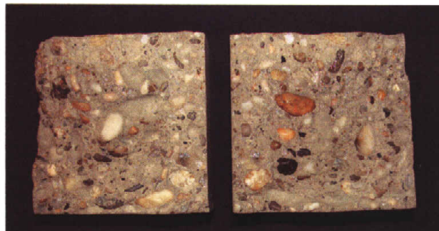
Figure 3 Pictures of fracture surface of young concrete on witch is not possible to measure penetration depths
