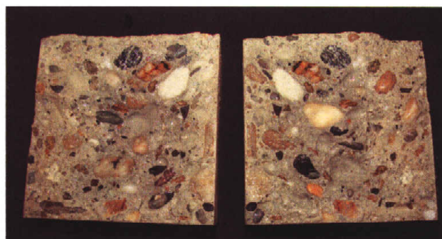
Figure 4 Pictures of fracture surface of no saturated aged concrete on witch are measured penetration depths
