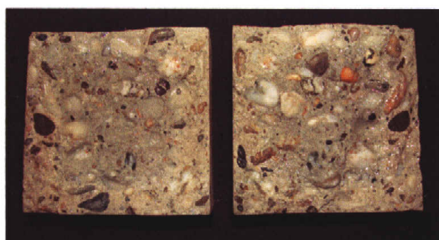
Figure 5 Pictures of fracture surface of saturated aged concrete on witch are measured penetration depths
