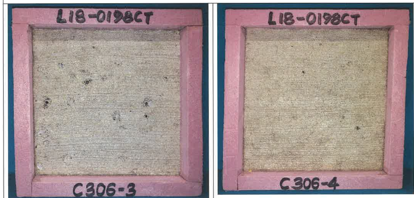
Slab C306-3 and Slab C306-4, Sealed test samples after completion of 25 freeze-thaw cycles.
